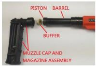
3. Pull barrel assembly out of housing. Unscrew muzzle cap. Pull buffer out of muzzle cap. Inspect and replace if buffer is worn.
