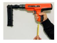
Insert the powder load strip from the end of handle until flush with the bottom. Always insert from the bottom of the tool and remove from the top.
