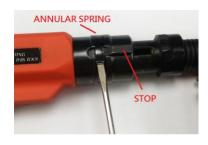
1. Using screw driver to lift end of annular spring and rotate toward the top of the tool so the stop is uncovered.
