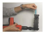
Insert the collated pins into the bottom of the magazine and move it as close to the top as possible.
