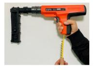
4. Insert the powder load strip from the end of handle until flush with the bottom. Always insert from the bottom of the tool and remove from the top.
